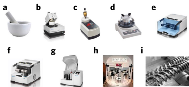
Fig. 3 Commonly used milling equipment. (a) Mortar and pestle, (b) automatic mortar, (c) vertical vibrational mini mill, (d) vibratory micro-mill, (e) vibrational ball mill, (f) vibrational ball mill with temperature control, (g) planetary ball mill, (h) multisampling mill, and (i) twin-screw for continuous mechanochemical synthesis. Reproduced with permission from ref. 15.
