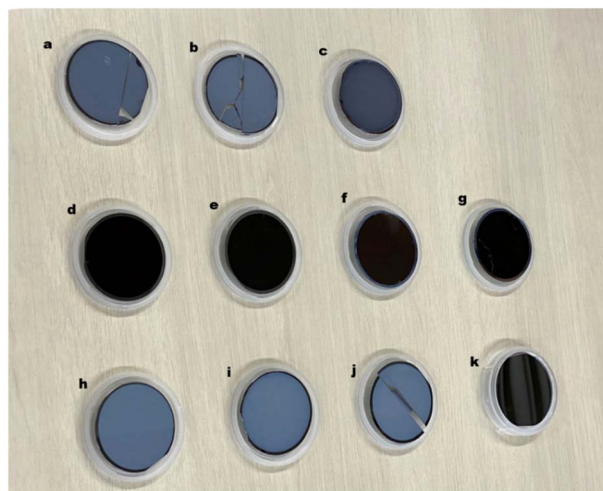
Fig. 5 (a)–(c) Samples grown at different substrate temperatures of 540, 520, and 480 °C, respectively. The sample grown at a substrate temperature of 480 °C has a darker surface, which suggests that the substrate temperature has an effect on the surface characteristics. (d)–(g) Samples grown under identical growth conditions at a substrate temperature of 500 °C to examine the reproducibility of the growth process. (h)–(j) Samples grown at a substrate temperature of 560 °C with half the Ga and As 4 fluxes to before, which correspond to 3.2 \times 10^{14} \text{ cm}^{-2} \text{ s}^{-1} , and variation of the growth conditions by (h) reducing the substrate temperature to 480 °C during the GaAs core growth. (i) Supply of catalyst Ga on the surface before initiating the GaAs core growth. 46 (j) Reduction of the As supply to one-third during the core growth. (k) Si(111) substrate.
