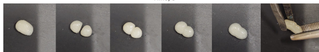
Fig. 8 Time-dependent self-healing of the hydrogel constructed of poly(1,2-epoxybutane- b -hyperbranched polyglycidol) at room temperature (at the top) and visual demonstration of the hydrogel reforming from two distinct pieces (at the bottom). The hydrogel sample was divided into two pieces. The fracture gradually vanished thanks to the self-healable properties of the 2-AAPBA-based boronic ester cross-links leading to its complete decay. The damaged hydrogel was completely repaired by regaining its initial mechanical properties.
