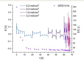
Fig. 5 Voltage traces (*E*-*t*) of galvanostatic plating of 1 mA h cm<sup>-2</sup> Li at increasing current densities between 0.2 and 3.2 mA cm<sup>-2</sup> in a Li symmetric cell, LP30 electrolyte and GF separator at RT. EIS intensity (purple spheres) measured with GEIS at 9 Hz with 100  $\mu$ A amplitude.
