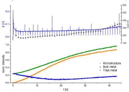
**Fig. 7** Operando <sup>7</sup>Li NMR and impedance (GEIS) measured at 8 Hz. Intensities measured during unidirectional Li plating at 0.5 mA cm<sup>-2</sup> in an NMR *in situ* cylindrical symmetrical Li cell with LP30 electrolyte.
