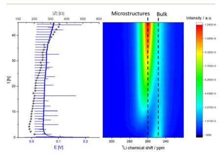
**Fig. 6** Operando NMR spectra of unidirectional Li deposition in an NMR *in situ* cylindrical symmetrical Li cell with LP30 electrolyte (right) with corresponding voltage profile and impedance (GEIS) intensity measured at 9 Hz (left) during galvanostatic plating with a current density of 0.5 mA cm<sup>-2</sup>.
