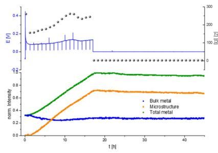
**Fig. 8** Operando <sup>7</sup>Li NMR and impedance (GEIS) measured at 8 Hz intensities measured during unidirectional Li plating at 1 mA cm<sup>-2</sup> in an NMR *in situ* cylindrical symmetrical Li cell with LP30 electrolyte.
