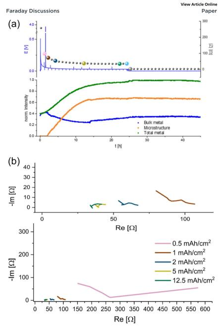
Fig. 9 (a) Operando <sup>7</sup>Li NMR and impedance (GEIS) measured at 9 Hz. Intensities measured during unidirectional Li plating at 1 mA cm<sup>-2</sup> in an NMR *in situ* cylindrical symmetrical Li cell with LP30 + 10% FEC electrolyte. (b) GEIS Nyquist plots measured with 100  $\mu$ A amplitude during Li plating at 1 mA cm<sup>-2</sup> in an NMR *in situ* cylindrical symmetric cell, using LP30 + FEC electrolyte with GF separator at RT. Magnification of the plot at 5–15 mA h cm<sup>-2</sup>.
