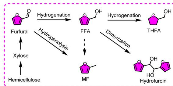
Fig. 10 Reaction pathways in the electroreduction of furfural.
