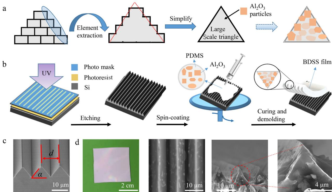
**Fig. 2** Design and preparation of the BDSS films. (a) The characteristic model extracted from the microstructure of the inner surface of the *Hawaiian scallop* shell. (b) The schematic diagram of the particle doping and polymer molding processes. (c) The SEM image of the silicon wafer template. (d) The optical and SEM images of the BDSS film.
