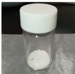
Fig. 9 A photograph of the Mg[TFSA] 2 sample after NH 3 absorption/desorption cycles at 300 K. Mg[TFSA] 2 sample in the glass bottle (ø 24 mm, 10 mL).
