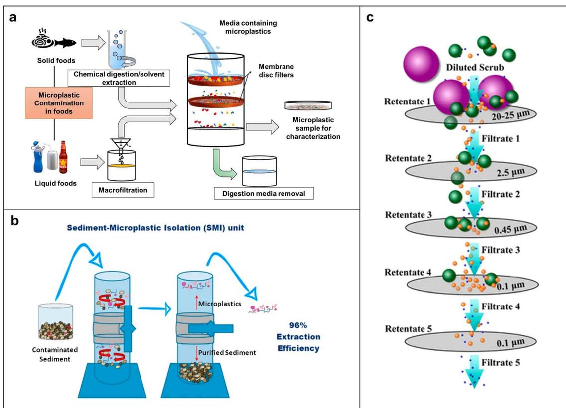
Fig. 3 Working principle of various filtration methods for MP separation. (a) Mechanistic scheme for the separation of MPs via membrane filtration. Reproduced with permission,<sup>77</sup> Copyright 2021, Elsevier. (b) Schematic of SMI. (c) Scheme of the filtration process with the complex mechanism. Reproduced with permission,<sup>84</sup> Copyright 2017, American Chemical Society.
