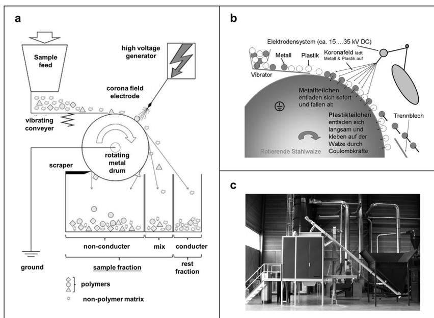
Fig. 7 Schemes of the mechanism and process for separation of MPs based on electrostatic interaction. (a) Schematic of the electrostatic separator. Reproduced with permission,<sup>97</sup> Copyright 2017, Elsevier. (b) Working mechanism of the corona roller separator type hamos KWS. Reproduced with permission,<sup>98</sup> Copyright 2019, Springer-Verlag. (c) Physical view of a KWS electrostatic separator (hamos 1521-1). Reproduced with permission,<sup>98</sup> Copyright 2019, Springer-Verlag.
