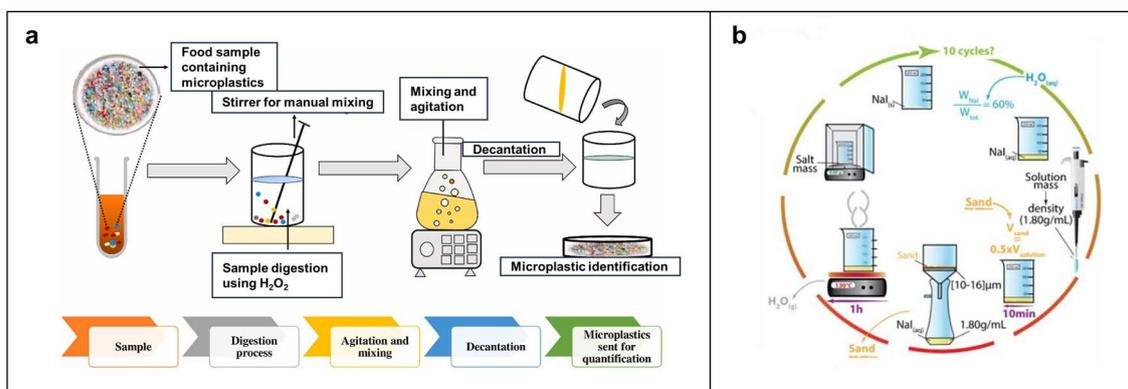
Fig. 2 Flow charts of MPs separation based on density flotation. (a) Basic flow of density flotation. Reproduced with permission,<sup>77</sup> Copyright 2021, Elsevier. (b) The detailed process of separating MPs via NaI-enabled density flotation. The recycling and reuse of NaI in the process can help reduce the cost and waste of the method. Reproduced with permission,<sup>78</sup> Copyright 2016, Elsevier.
