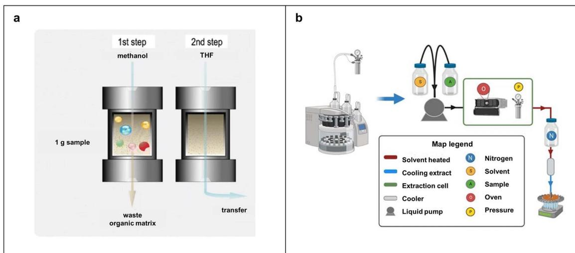
**Fig. 6** Pressurized liquid extraction methods for the separation of MPs. (a) Basic flow of pressurized fluid extraction method. Reproduced with permission,<sup>94</sup> Copyright 2019, Springer-Verlag GmbH Germany, part of Springer Nature. (b) Schematic of pressurized liquid extraction equipment and the operation flow.
