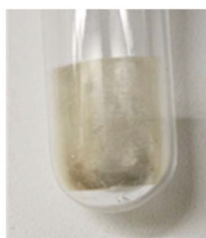
Fig. 3 Photograph of the deposited powder after photolysis of oligo(3,4-di-iso-propylsilacyclopentene) ( OligoSi ) in THF.
