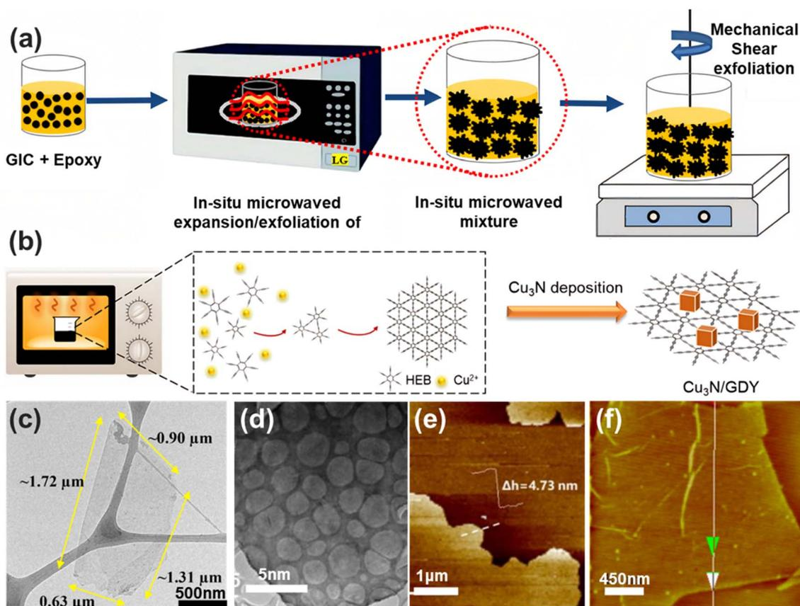
Fig. 7 (a) Schematic for preparation of epoxy/graphene nanocomposites. (b) Schematic illustration of the synthesis of  $\text{Cu}_3\text{N}$ /GDY. (c) TEM images of graphene platelets. (d) TEM and (e) AFM images of GDY. (f) Typical AFM height images of MW-rGO.
