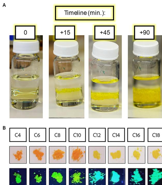
**Fig. 1** (A) Images taken during the synthesis of poly-crystals with long ligands ( $C \geq 12$ ) growing in the interphase between methanol and HI. (B) Images of the obtained poly-crystals under white light, and under UV light (bottom).
