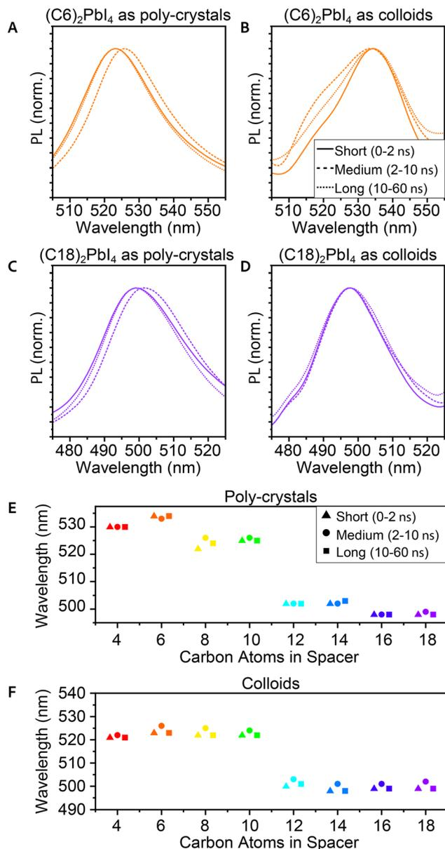
**Fig. 4** TRPL of the 2D  $(C_n)_2PbI_4$  MHP in 3 time frames of the PL decay – 0–2 ns, 2–10 ns, and 10–60 ns. (A)  $(C_6)_2PbI_4$  as poly-crystals, and (B) as colloids. (C)  $(C_{18})_2PbI_4$  as poly-crystals, and (D) as colloids. (E) Comparison of the PL peak wavelengths at the different time frames of poly-crystals and (F) colloids.
