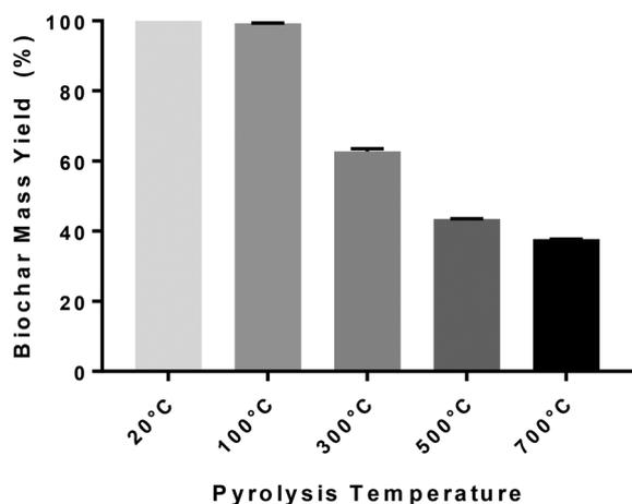
**Fig. 1** Impact of pyrolysis temperature on biochar mass yield. Bars represent the average yield and error bars represent the standard deviation among triplicate experiments ( $n = 3$ ).
