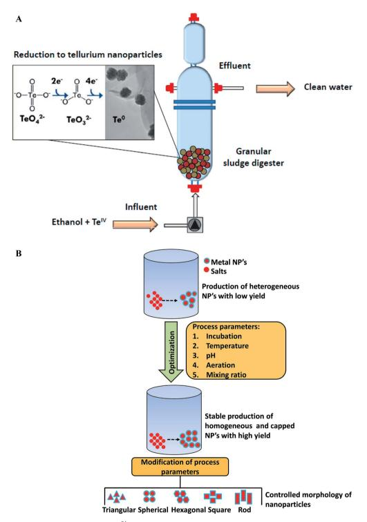
**Fig. 5** (A) Continuous reduction of toxic tellurite (Te<sup>IV</sup>) oxyanions into recoverable tellurium nanoparticles using anaerobic sludge reactor [this figure has been adapted from ref. 153 with permission from Elsevier]; (B) parameters for producing monodispersed, stable, and high-yield biological nanoparticles [this figure has been adapted from ref. 16 with permission from Elsevier].
