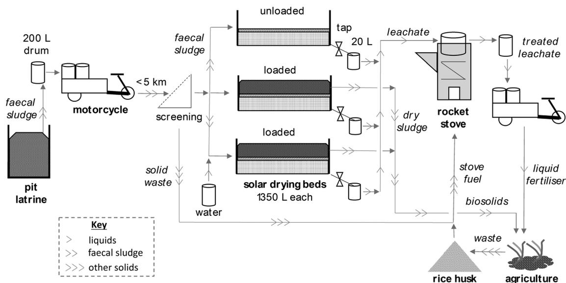
**Fig. 3** Process flow diagram for the faecal sludge treatment system. The flows through the system are separated into: liquids (single arrow), faecal sludge (double arrows) and other solids (triple arrows). The top drying bed is in an unloaded state to indicate how the treatment system was batch operated.
