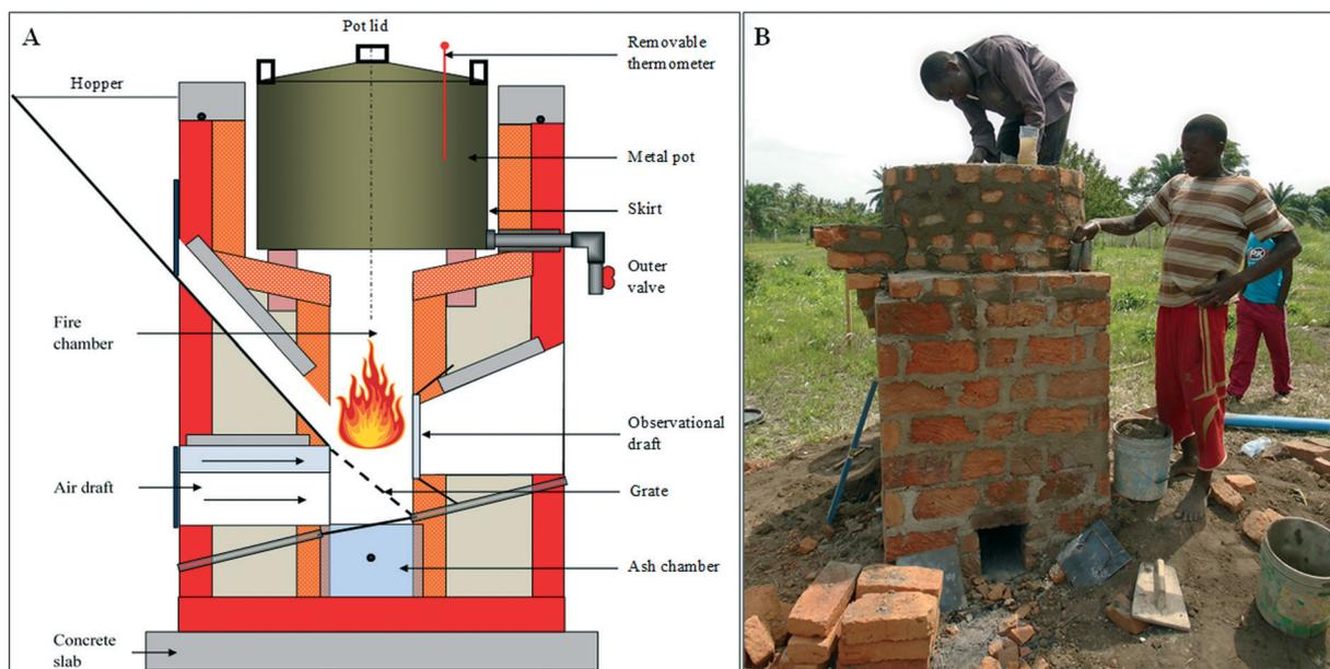
Fig. 2 Rocket stove A. Design schematic. B. Construction using local materials and labor in Kining'ina, Tanzania.
