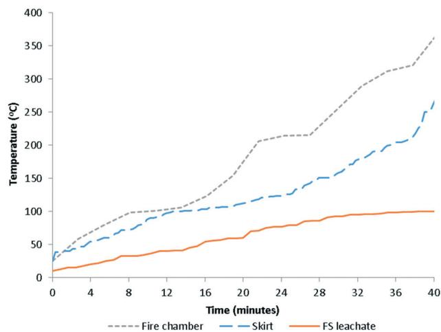
Fig. 4 Heat sterilisation temperature profiles of faecal sludge leachate using rocket stove fired with agricultural waste.
