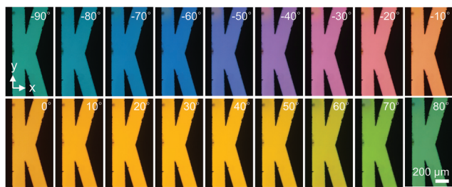
Fig. 5 Anti-counterfeiting code made of HNF film. Color variation of security letter "K" in various polarization conditions.
