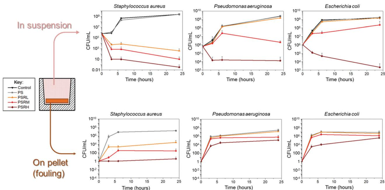
**Fig. 12** Bacterial growth curves (CFU counting) for *S. aureus*, *P. aeruginosa* and *E. coli* in contact with all formulations of hybrids. Cells in suspension (top) and attached to the samples (bottom) were both counted. Empty culture wells with  $\alpha$ MEM were used as negative control when relevant.
