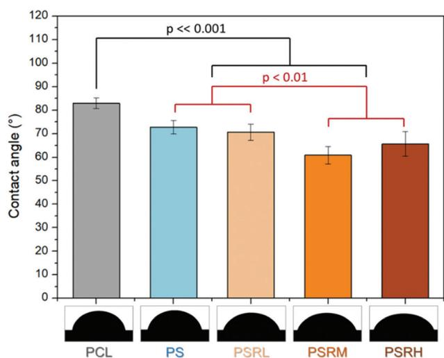
Fig. 5 Droplet profiles and contact angle measurements for all formulations of PCL/silica tested ( $n = 3$ ). Note the effect of both the introduction of silica gel ( $p \ll 0.001$ ) and of rifampicin ( $p < 0.01$ ) on the hydrophilicity of the samples.
