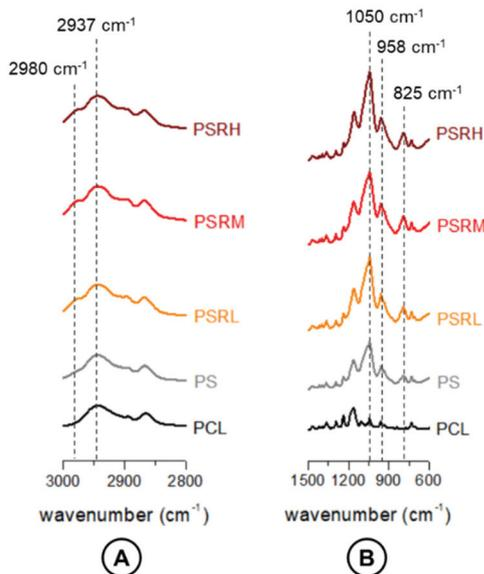
Fig. 8 (A) FTIR spectra highlighting the appearance of a new peak at 2980  $\text{cm}^{-1}$  in correspondence of the stretching vibration of C–H following the addition of rifampicin. (B) FTIR spectra comparing the 1500–900  $\text{cm}^{-1}$  range before and after sol–gel synthesis. Note the carbon–oxygen ester stretching of PCL at 1170  $\text{cm}^{-1}$  and the appearance of peaks associated with silica gel: Si–O–Si (1050 and 825  $\text{cm}^{-1}$ ) and Si–OH (958  $\text{cm}^{-1}$ ).
