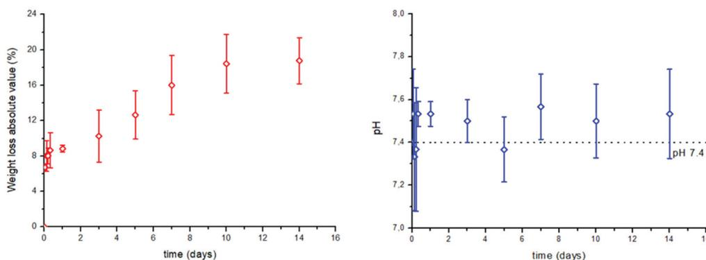
Fig. 6 Graphs showing a typical trend for weight loss (left) and pH (right), following immersion in culture medium for PCL/silica hybrids (results for PSRM are shown, other samples are comparable). The measurements are not affected by the addition of rifampicin: no statistically significant variation was observed varying the concentration of antibiotic ( $p > 0.05$ , see ESI†).
