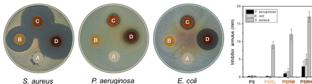
Fig. 11 Images of a typical agar diffusion assay of PS (A), PSRL (B), PSRM (C) and PSRH (D) samples against *Staphylococcus aureus*, *Pseudomonas aeruginosa* and *Escherichia coli*. On the graph on the right, a quantification of the inhibition width is reported.
