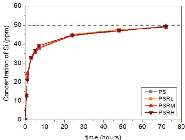
**Fig. 9** Silicon release from PCL/silica hybrids immersed in  $\alpha$ MEM. As expected, concentrations measured by ICP-OES do not vary depending on the rifampicin content.
