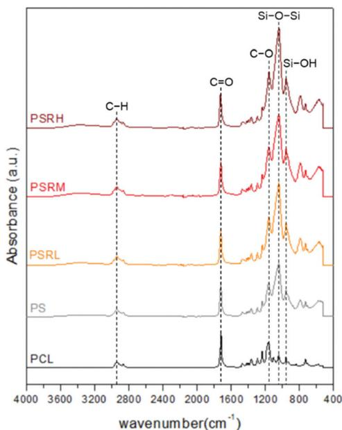
Fig. 7 Comprehensive FTIR spectra (4000–400  $\text{cm}^{-1}$ ) of PCL (bottom) and the four formulations of PCL/silica hybrids tested in our study. The major characteristic peaks of PCL (C–H, C=O, C–O), silica gel (Si–O–Si, Si–OH) and rifampicin (C–H) are highlighted. All spectra are normalized with respect to the characteristic peak of PCL at 1720  $\text{cm}^{-1}$ .
