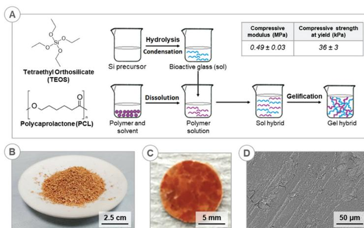
**Fig. 4** Schematic representation of the synthesis procedure (A). The inset shows typical mechanical parameters for this type of hybrid taken from ref. 26. Pictures of the material (PSRM, in this case) are also presented: powder (B) and pellet (C) forms are both shown. An SEM micrograph (D) of the same pellet can be also observed (magnification 300 $\times$ ).
