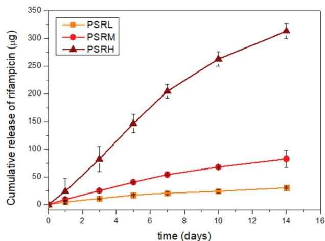
**Fig. 10** Cumulative release of rifampicin from all the formulations of tested samples. The antibiotic content in the medium is dependent on the loaded amount, confirming that this technology can be used to tailor rifampicin release.
