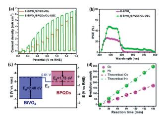
Fig. 11 (a) J-V curves of E-BiVO<sub>4</sub>/BPQDs/OL and E-BiVO<sub>4</sub>/BPQDs/ OL-OEC. (b) IPCE values of E-BiVO<sub>4</sub> and E-BiVO<sub>4</sub>/BPQDs/OL-OEC. (c) Band alignment diagram of E-BiVO<sub>4</sub> and BPQDs showing type II heterojunction. (d) HER and OER activities of the E-BiVO<sub>4</sub>/BPQDs/OL-OEC photoanode at 1.23 V vs. RHE. Reproduced with permission from ref. 133 © 2022 The Royal Society of Chemistry.
