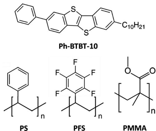
Fig. 1 Chemical structures of the employed small molecule organic semiconductor (top) and the binding polymers (bottom).
