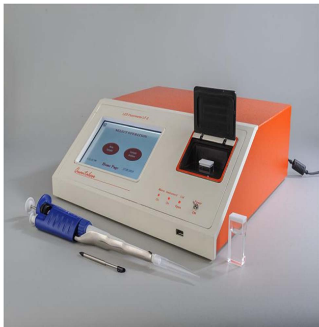
Fig. 2 LED fluorimeter (model LF-2) (QUANTALASE, India).
