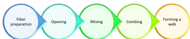
Fig. 3 Steps involved in the formation of nonwovens.
