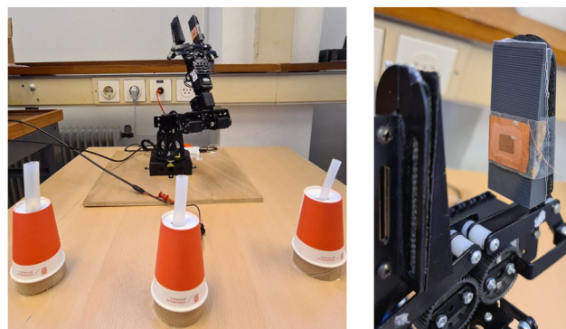
Fig. 6 Setup for tactile sensing experiment on robot arm.
