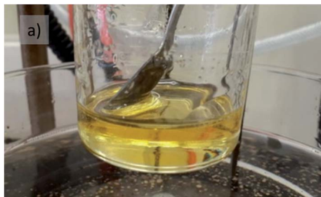
Fig. 1 (a) Liquid monosaccharide-urea melt obtained from glucose.
