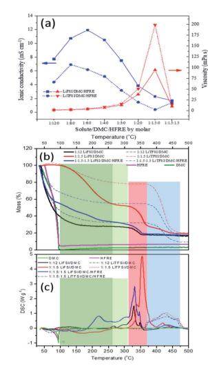
**Fig. 3** The ionic conductivities (blue, left *y*-axis) and viscosities (red, right *y*-axis) (a) of LiTFSI : DMC : HFRE and LiFSI : DMC : HFRE electrolytes at different molar ratios. The TGA (b) and DSC (c) curves of electrolytes with various concentrations and solvents.
