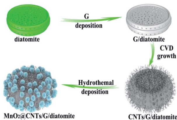
Fig. 8 Illustration of the \text{MnO}_2 @CNTs/G/diatomite composite fabrication. 105
