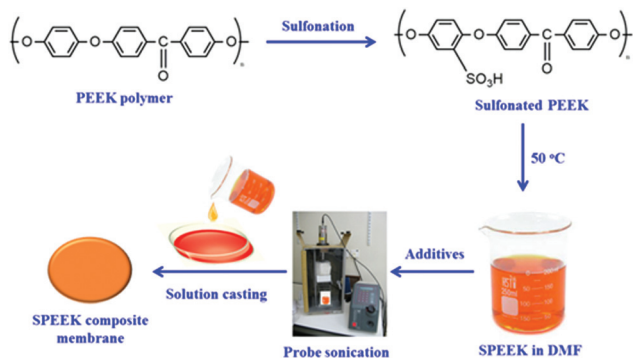
Fig. 5 Schematic preparation of SPEEK membranes.
