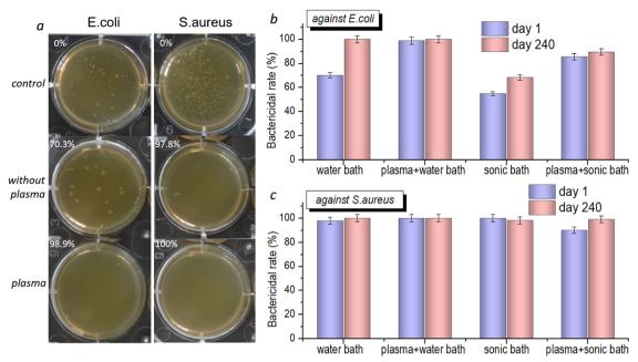
Fig. 6 (a) Images and percentage antibacterial activity of dyed fabrics (3% mordant coated in a water bath) with and without plasma treatment and (b, c) antibacterial shelf life of dyed cotton measured after day 1 and day 240.
