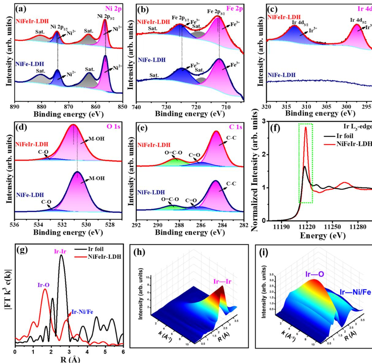
Fig. 3 XPS spectra of the as-synthesized NiFe-LDH and NiFeIr-LDH nanosheets: (a) Ni 2p, (b) Fe 2p, (c) Ir 4d, (d) O 1s and (e) C 1s. (f) Ir  $L_{3}$ -edge XANES spectra and (g) the corresponding Fourier transforms of Ir  $L_{3}$ -edge EXAFS spectra of the as-synthesized NiFeIr-LDH nanosheets and the standard reference Ir foil. Wavelet transforms of the EXAFS signals for the (h) standard reference Ir foil and (i) NiFeIr-LDH nanosheets.
