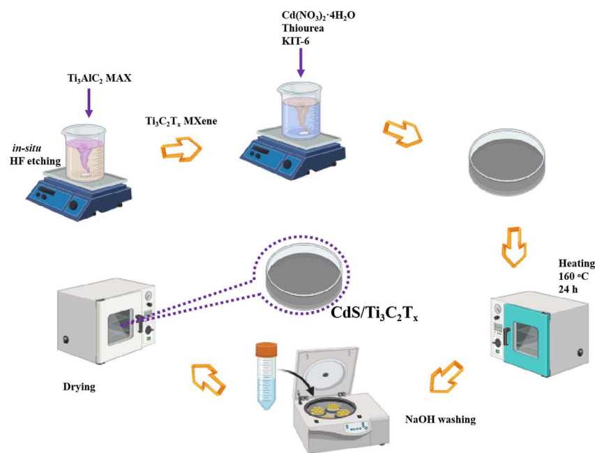
Fig. 1 Synthesis of \text{CdS}/\text{Ti}_3\text{C}_2\text{T}_x composites (schematic).
