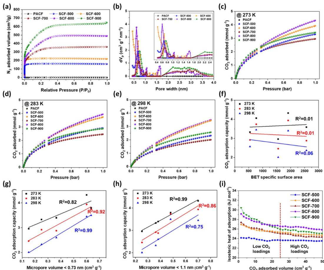
Fig. 4 (a)  $N_2$  adsorption–desorption isotherms of the prepared samples at 77 K; (b) pore size distribution; (c–e)  $CO_2$  adsorption–desorption isotherms at 273, 283, and 298 K, and the correlations between the  $CO_2$  adsorption capacity and textural properties at different temperatures: 273, 283, and 298 K; (f) BET specific surface area with different pore size ranges less than (g) 0.73 and (h) 1.1 nm; (i) isosteric heat of adsorption for the prepared samples.
