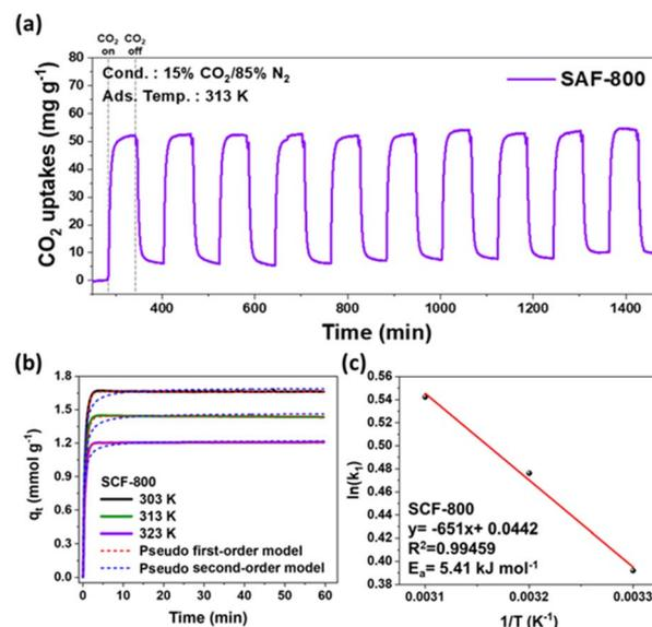
**Fig. 5** (a) CO<sub>2</sub> adsorption–desorption profiles over 10 continuous vacuum swing adsorption cycles of SCF-800 under flue gas conditions (15% CO<sub>2</sub>/85% N<sub>2</sub> gas mixture) at 313 K. (b) Kinetic study of CO<sub>2</sub> adsorption in SCF-800. (c) Pseudo first-order adsorption rate constant-based Arrhenius plot for estimating the activation energy.
