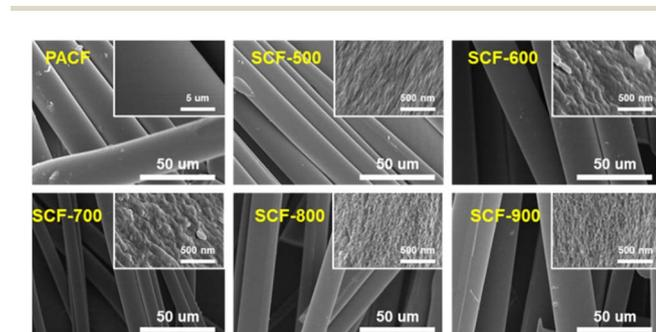
Fig. 2 High-resolution scanning electron microscopy image of the PACF and SCF samples.
